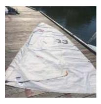
2) Fold the top of the main sail at its upper batten (rigid section):
