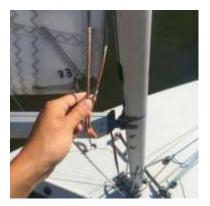
11)Pull the cunningham to bring the eye of the corner of the main sail close to the boom. Then, you will be able to feed the pin hanging from the boom onto the eye of the corner of the main sail.
