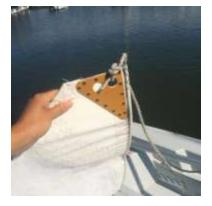
5) Insert the top of the main sail in the track of the mast.
