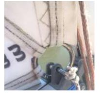
12) Hook the boom to the shroud furthest to the dock. It will clear the air to allow a sailor to transfer safely into the boat:
